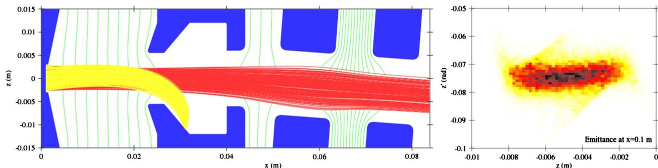
FIG. 3. (Color online) 3D simulation of  $H^-$  LEPT with 12 keV final beam energy. The coextracted electron beam is deflected into a water-cooled electron dump by a magnetic filter at the energy of 6 keV. The ion beam is symmetric and has little aberrations at the end of the simulation.
